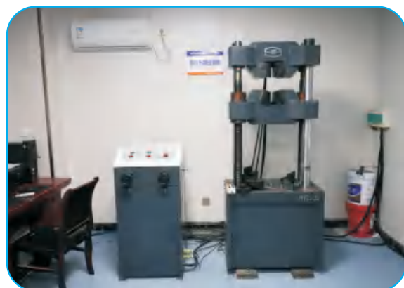
液压万能试验机 Hydraulic universal testing machine
