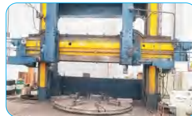
2×φ6.3米数控立车 φ 6.3 m CNC vertical lathe
