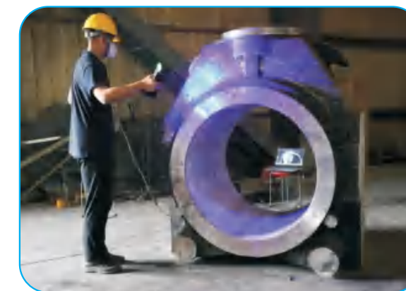
三维扫描 Three-dimensional scanning
