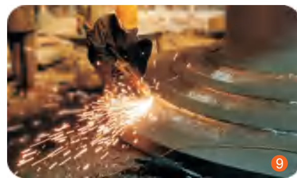
精整打磨 Finishing
