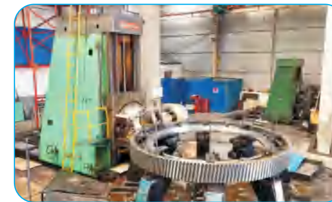
3×φ8米滚齿机 φ8m gear hobbing machine
