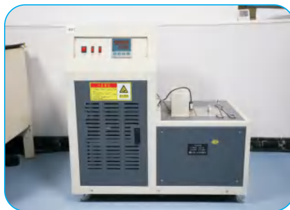
冲击试样低温槽 Impact test specimen low-temperature bath
