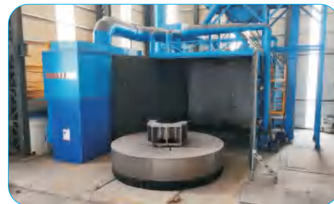
8米 × 8米全自动台车式抛丸机 8m x 8m Fully automatic trolley type shot blasting machine
