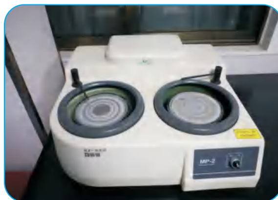
金相试样磨抛机 Metallographic sample grinding and polishing machine
