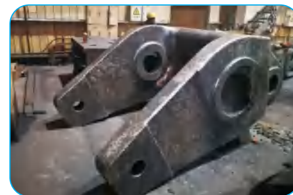
摇臂 Vertical mill rocker arm
