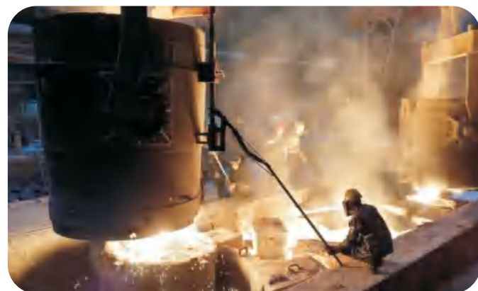
双包浇注 Double-ladle casting
