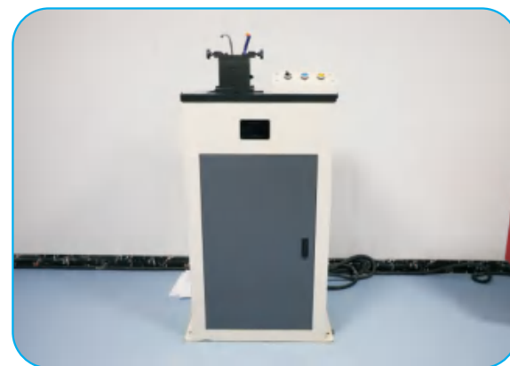
冲击试样缺口拉床 Impact specimen notch broaching machine
