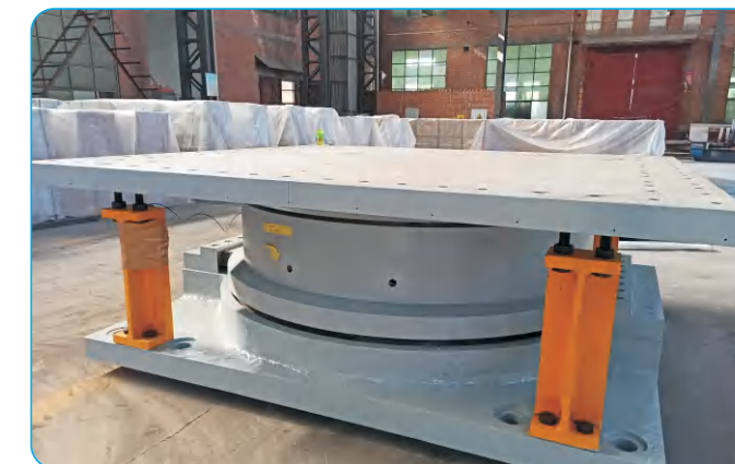
( 澳门澳氹大桥 ) 桥梁支座板 (Macao Cotai Bridge) bridge support plate
