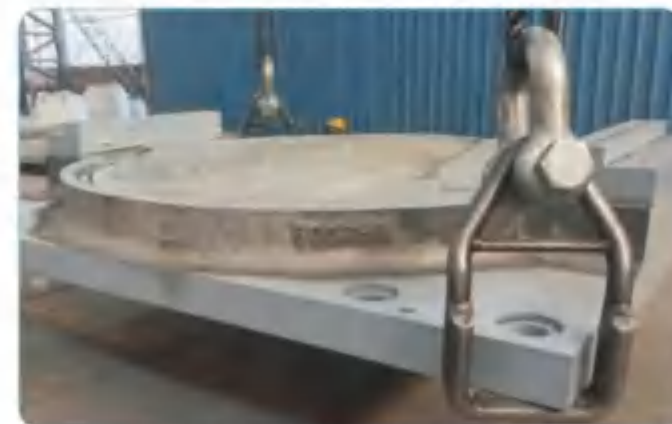
不锈钢支座板 (材质316L) Stainless support plate (material 316L)
