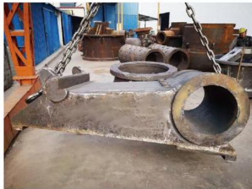
动臂 Vertical mill swing arm
