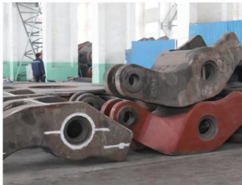
摇臂 Vertical mill rocker arm
